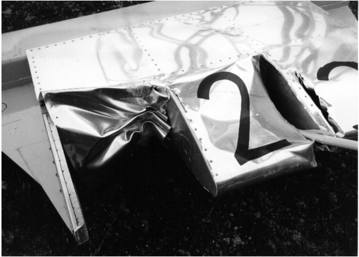
Figure A1.11 The unique failure mode of this test is clearly visible. The front spar was not damaged despite the cut rivets.
