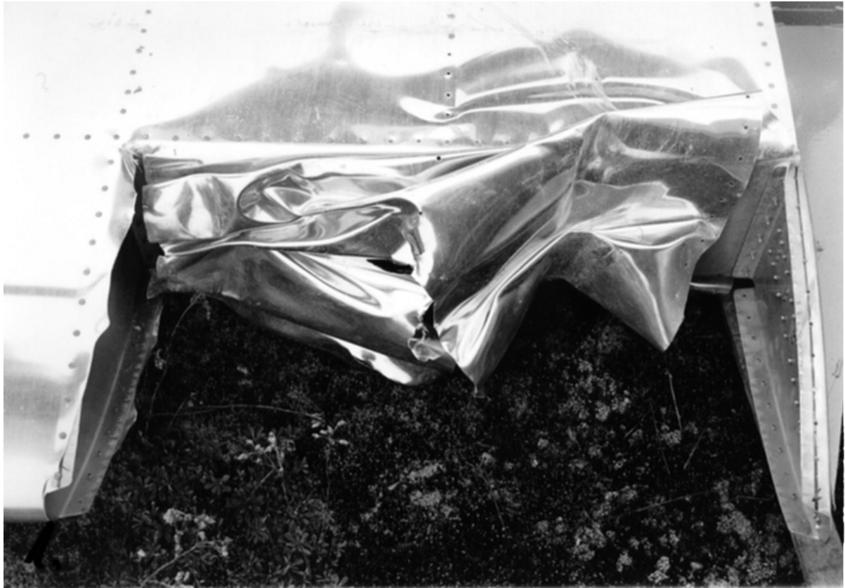
Figure A1.5 The damages caused to the wing are clearly visible in this picture. The 0.8 mm skin has been torn and crushed, but the front spar has not been touched. The only damages further back are the small buckle in the rightmost panel and three loose rivets (rib/skin joint in the middle).
