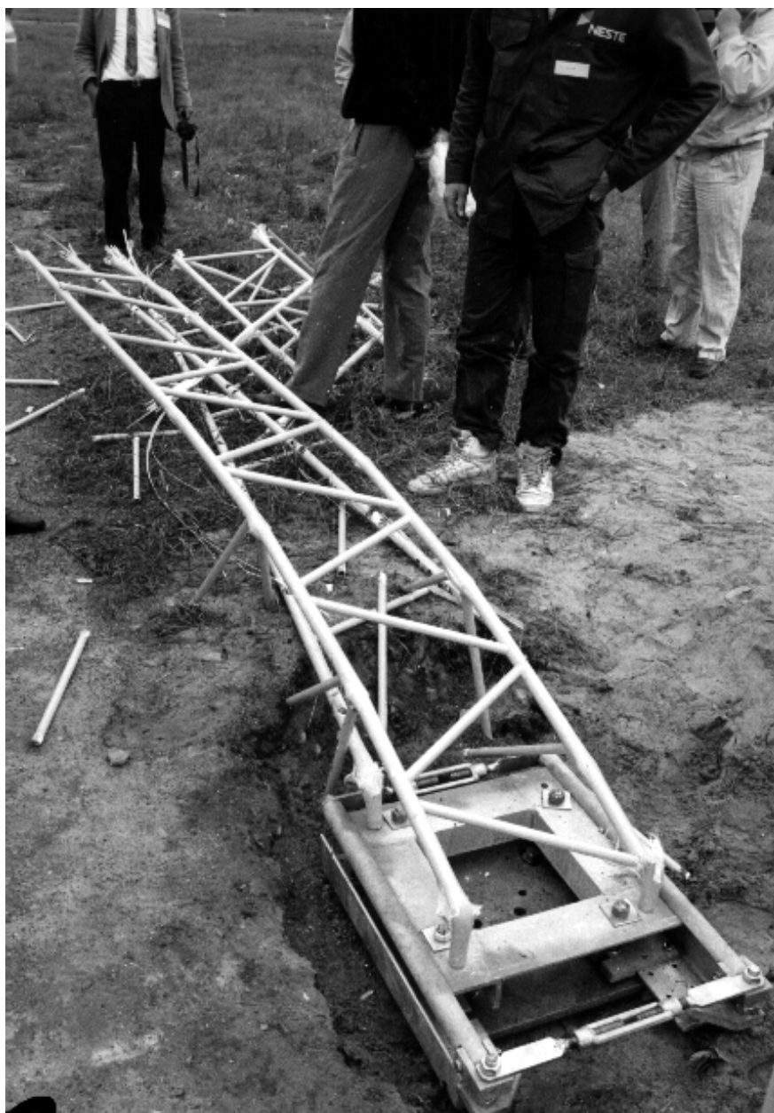
Figure A1.14 The mast was cut through by the impactor. The upper part broke into several parts and the lower section suffered a total collapse when the vertical tubes were bent at the root and most of the diagonals came loose. This is a very good example of the frangible behaviour of the masts.
