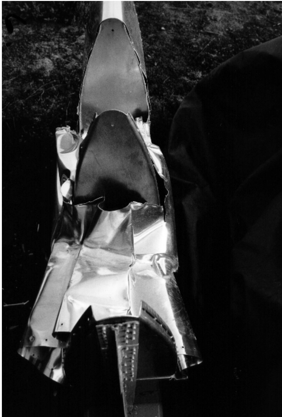
Figure A1.23 Side view of the damaged wing. Damages are very similar to those of tests 1 and 5. The behaviour of the mast was almost identical to the test 5 (not shown).
