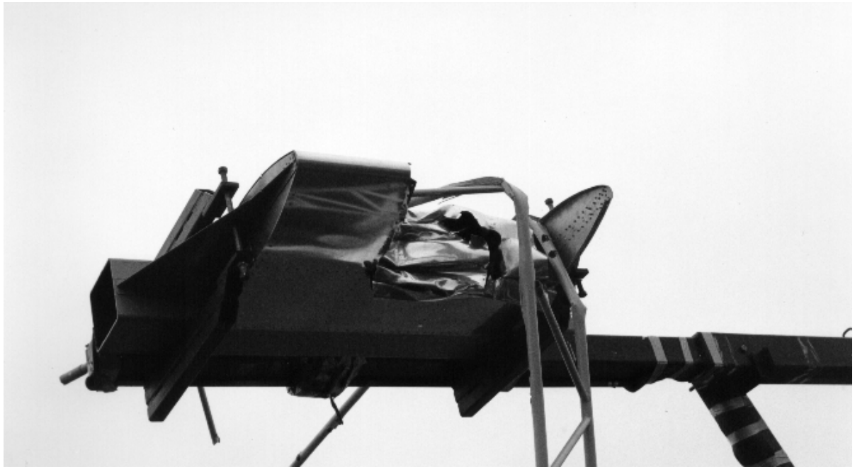
Figure A1.3 Test wing section immediately after the impact. Part of one side of the mast remained hanging from the wing. In this case it was completely loose, it did not get stuck. Note that the penetration has stopped at the front spar and that in the outmost rib section even the thin skin panels remain undamaged.
