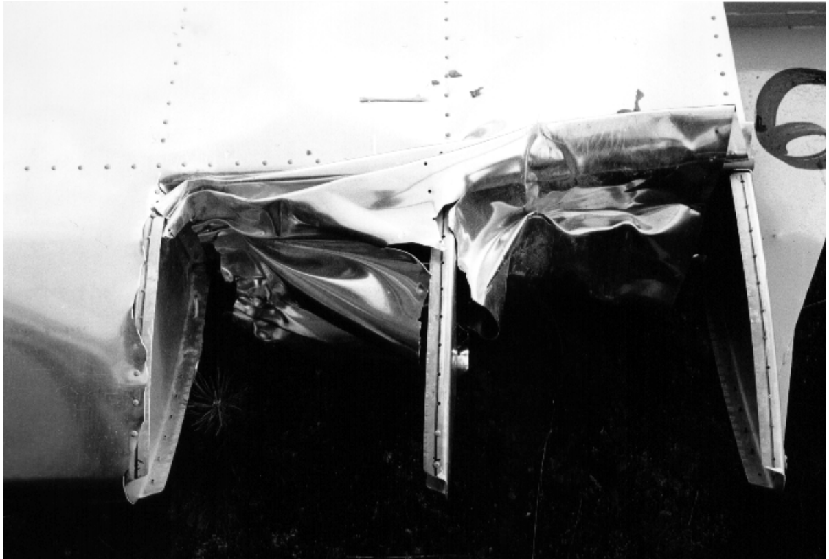
Figure A1.24 As seen already from the previous picture this a very typical example of the wing section of these tests: two crushed leading edge sections, the next rib section in perfect condition and the front spar intact. It is obvious that an aircraft with this kind of damage would still be able to fly. The fact that this wing section suffered the highest impact energy, could not be detected in the post-impact inspection.
