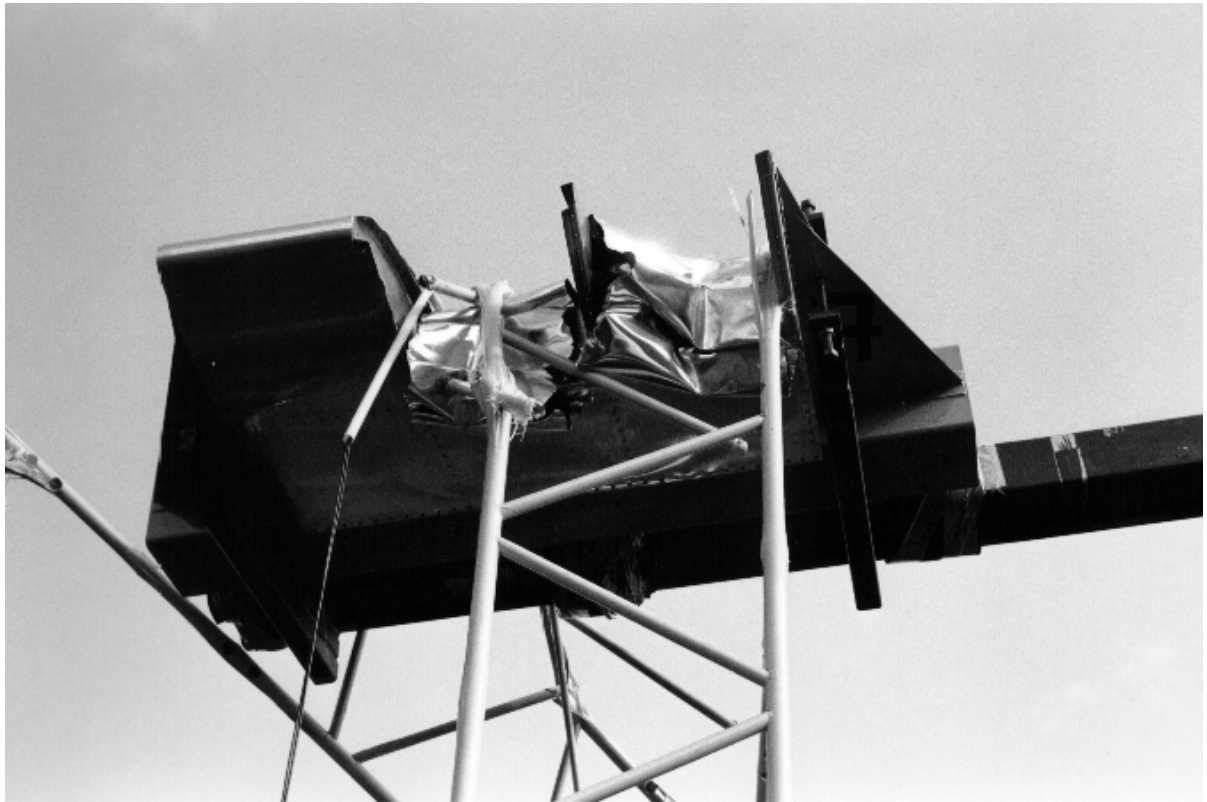
Figure A1.27 In test 7 the mast structure acted like in tests 5 and 6 but the cables and the cover tube failed to cut. In this test they were located at the side of the impact. From the high speed camera recording it can be seen that this is also the side of compressive loading, which is a possible reason to this cable behaviour. It can be seen that again it was the "rear" plane of the lattice structure that bent around the wing section.
