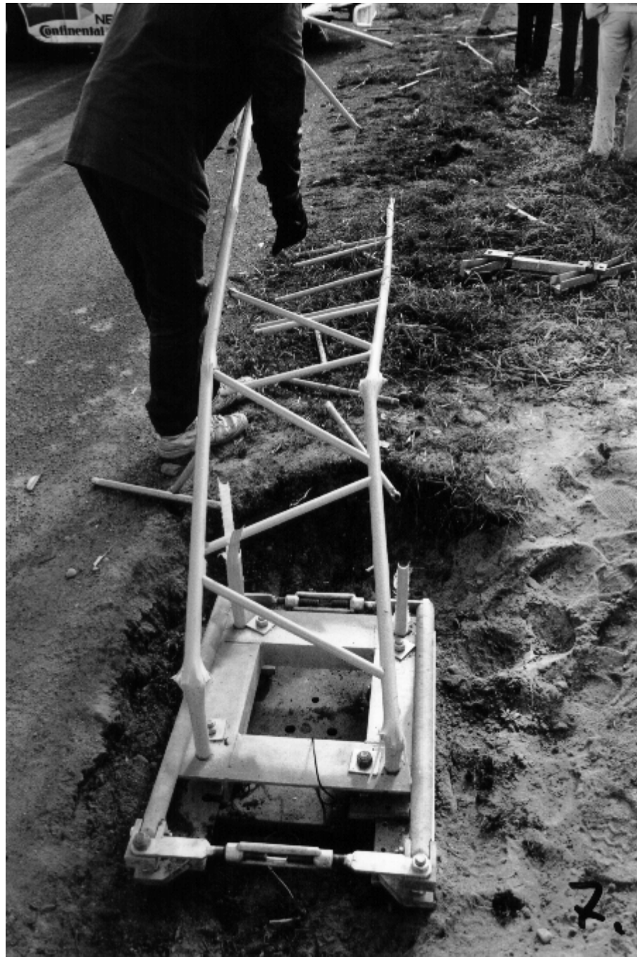
Figure A1.28 The lower section of the broken mast was left somewhat shorter in this test. The mast top weight is again visible in the upper right corner.
